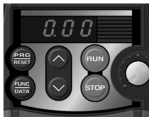
Figure 4.2 Display of the LED Monitor after Power-on
