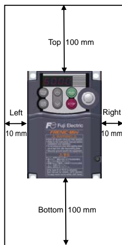
Figure 2.1 Mounting Direction and Required Clearances
