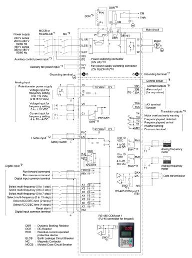
\*1 Install a recommended molded case circuit breaker (MCCB) or residual-current-operated protective device (RCD)/earth leakage circuit breaker (ELCB) (with overcurrent protection function) in the primary circuit of the inverter to protect wiring. Ensure that the circuit breaker capacity is equivalent to or lower than the recommended capacity.
