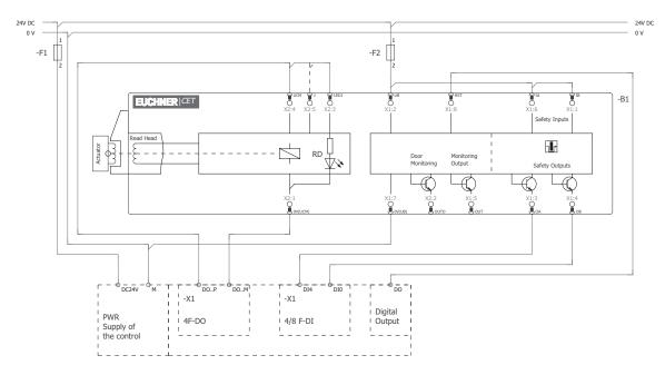
Fig. 7: Wiring diagram B, CET 3/4-AR with plug connectors 2 x M12 Dual-channel control of the guard locking solenoid
