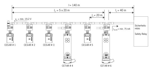
Fig. 3: Circuit example with six CES-AR/CET-AR
