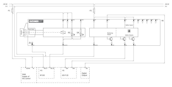
Fig. 11: Wiring diagram D, CET 1/2-AR with plug connector M23 Dual-channel control of the guard locking solenoid
