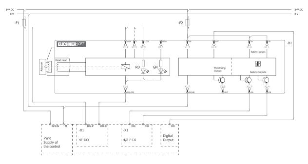
Fig. 5: Wiring diagram A, CET 1/2-AR with plug connectors 2 x M12 Dual-channel control of the guard locking solenoid
