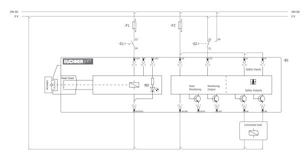
Fig. 6: Wiring diagram B, CET 3/4-AR with plug connectors 2 x M12 Single-channel control of the guard locking solenoid
