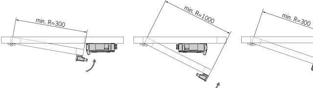
Fig. 2: Installation situation and door radii
