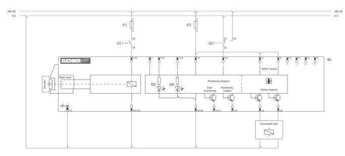
Fig. 12: Wiring diagram E, CET 3/4-AR with plug connector M23, versions with and without teach-in input Single-channel control of the guard locking solenoid
