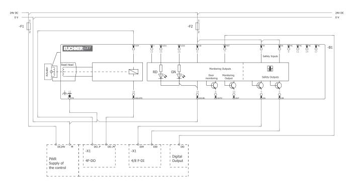
Fig. 13: Wiring diagram E, CET 3/4-AR with plug connector M23, versions with and without teach-in input Dual-channel control of the guard locking solenoid
