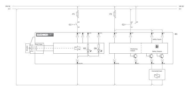
Fig. 4: Wiring diagram A, CET 1/2-AR with plug connectors 2 x M12 Single-channel control of the guard locking solenoid
