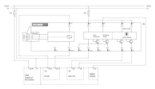
Fig. 9: Wiring diagram C, CET 3/4-AR with plug connectors 2 x M12 and additional monitoring output OUT Dual-channel control of the guard locking solenoid
