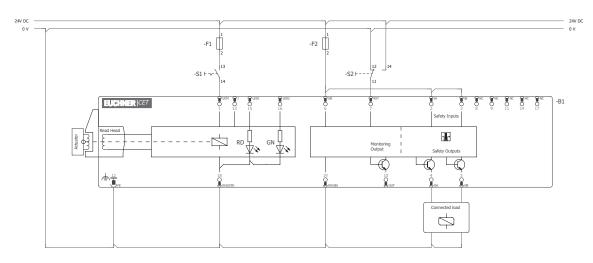
Fig. 10: Wiring diagram D, CET 1/2-AR with plug connector M23 Single-channel control of the guard locking solenoid
