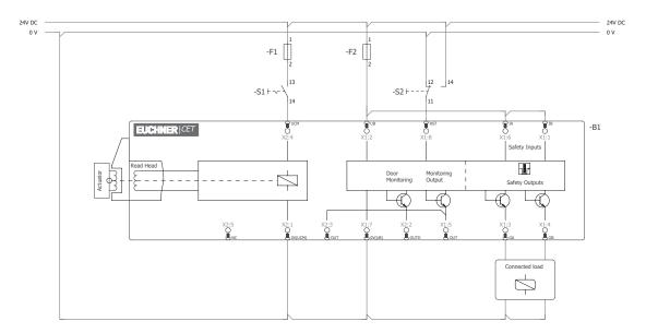
Fig. 8: Wiring diagram C, CET 3/4-AR with plug connectors 2 x M12 and additional monitoring output OUT Single-channel control of the guard locking solenoid
