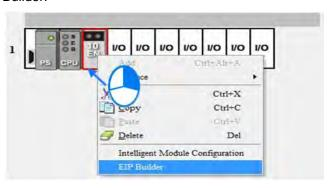
7.2 Right-click the AHCPU5x1-EN on the CPU's main backplane and you will see the EIP Builder. Double click it to open the EIP Builder.
