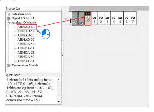
Add the I/O modules according to the real placement by dragging the modules on the left hand side to the right side of the RTU module. Make sure the slot assignment is the same as the real placement.
