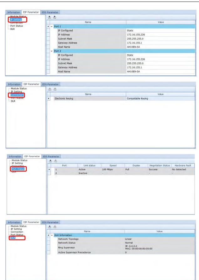
(c) EDS Parameter Tab: this is not supported on the AH10EN-5A series.
