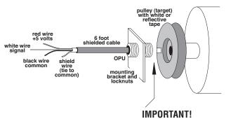
Optical pick-up face must be 1/8" to 1" from white marked surface or 3/8" to 4" from reflective marked surface!
