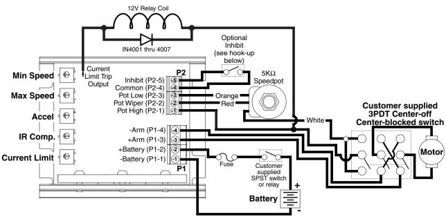
Caution: When reversing a spinning motor, care must be taken that the resulting current through the armature of the motor does not exceed the overload ratings of the control, or the demagnetize rating of the motor being reversed when using a permanent magnet DC motor.
