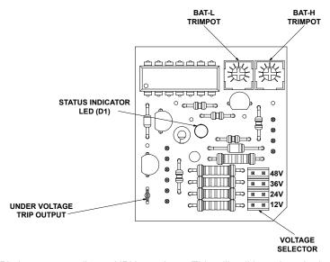
The Under Voltage Trip Pin is an open collector NPN transistor. This will pull low when the input Voltage goes below the Under Voltage Trip Point and stays low until the input Voltage goes above the Auto Reset Voltage Point. This output is rated to 50VDC at 150mA.
