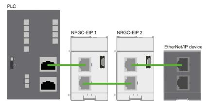
Fig. 3 Example of a line configuration of the NRGC-EIP with other EtherNet/IP devices and controller
