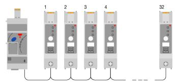
In case of an RG..N replacement, or any changes to the NRG bus chain, the RG..Ns have to be re-addressed. Follow the procedure below to re-address the RG..Ns on the NRG bus chain manually. Alternatively, auto-addressing can be done via an 'Explicit' command (check NRG EtherNet/IP User Manual for further information)
