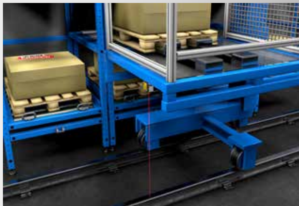
Positioning a storage and retrieval machine
