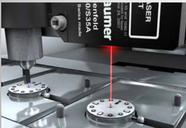
Precise positioning in watch manufacture Before the watch hand is mounted on the mandrel, a measurement of the distance to the hand shaft is carried out to prevent damage.
