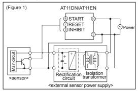
As (Figure 2), if using terminal ® as common terminal of input signal, it may cause damage to inner circuit of AT11DN/EN timer. Use terminal @ as common terminal referring to (Figure 3).
