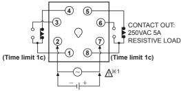
\*\*1: AC/DC voltage: 100-240VAC 50/60Hz, 24-240VDC : 24VAC 50/60Hz, 24VDC
