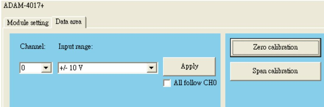
4. You may start calibrating by select "Zero Calibration". A pop-out window will be shown by telling you to apply 0.0V to the Channel 0
