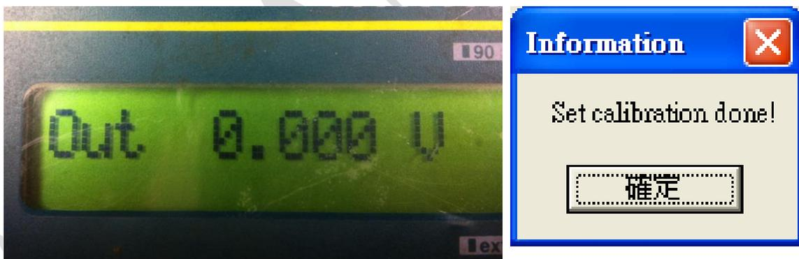
6. Similarly, you may execute SPAN calibration by click "SPAN Calibration", and apply 10.0V to the channel from power source.
